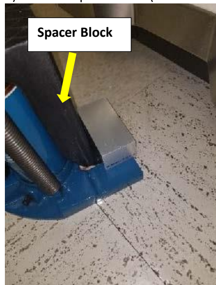
Figure 276: Placement of space block
