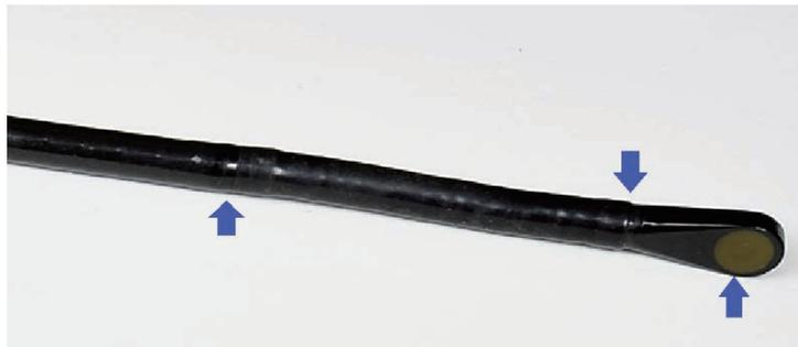
[Figure 1. TEE probe MMPT3-7 with contamination spots (arrows)]
